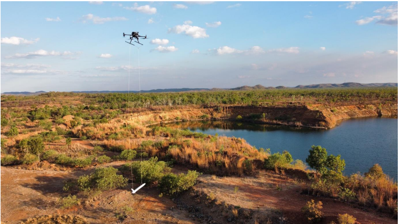
Figure 4: Drone-mag survey at Fountain Head
