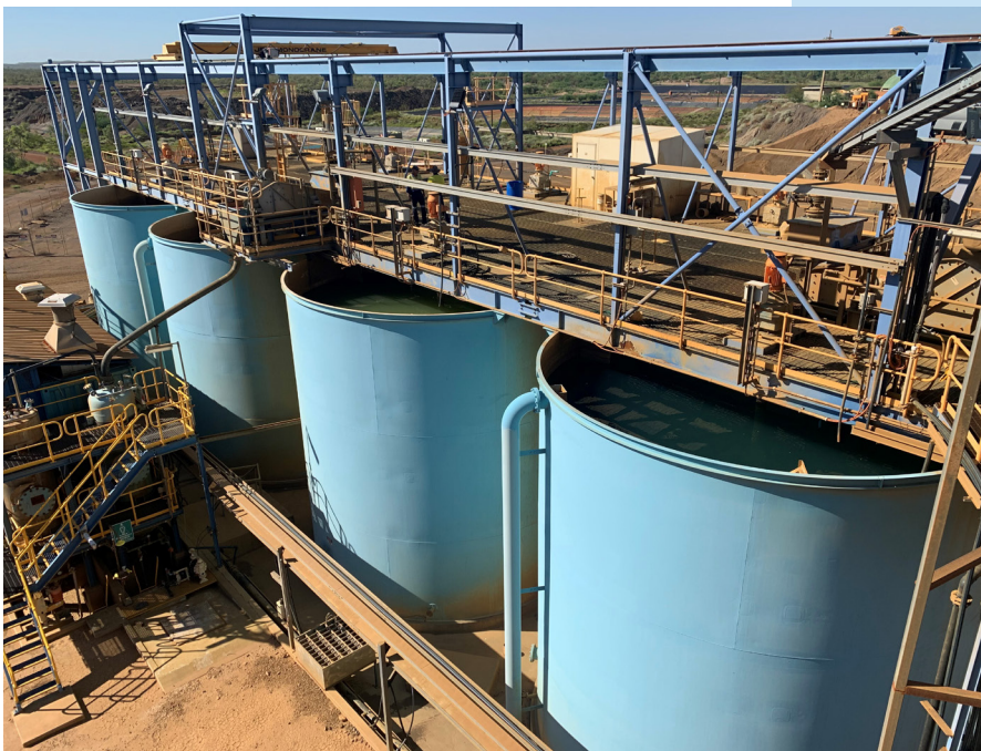
Figure 2 Typical carbon-in-leach tanks.
