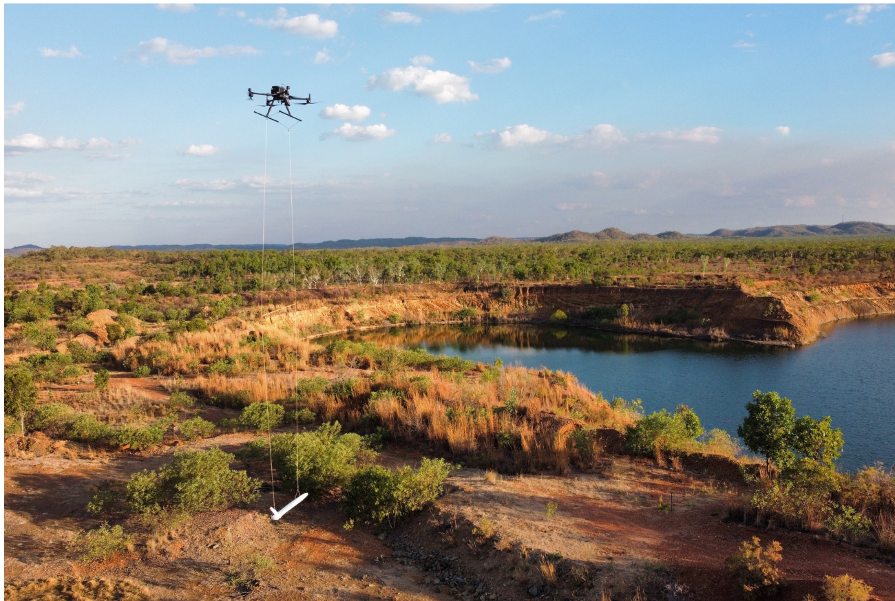
Figure 8 Drone magnetic survey at Fountain Head.
