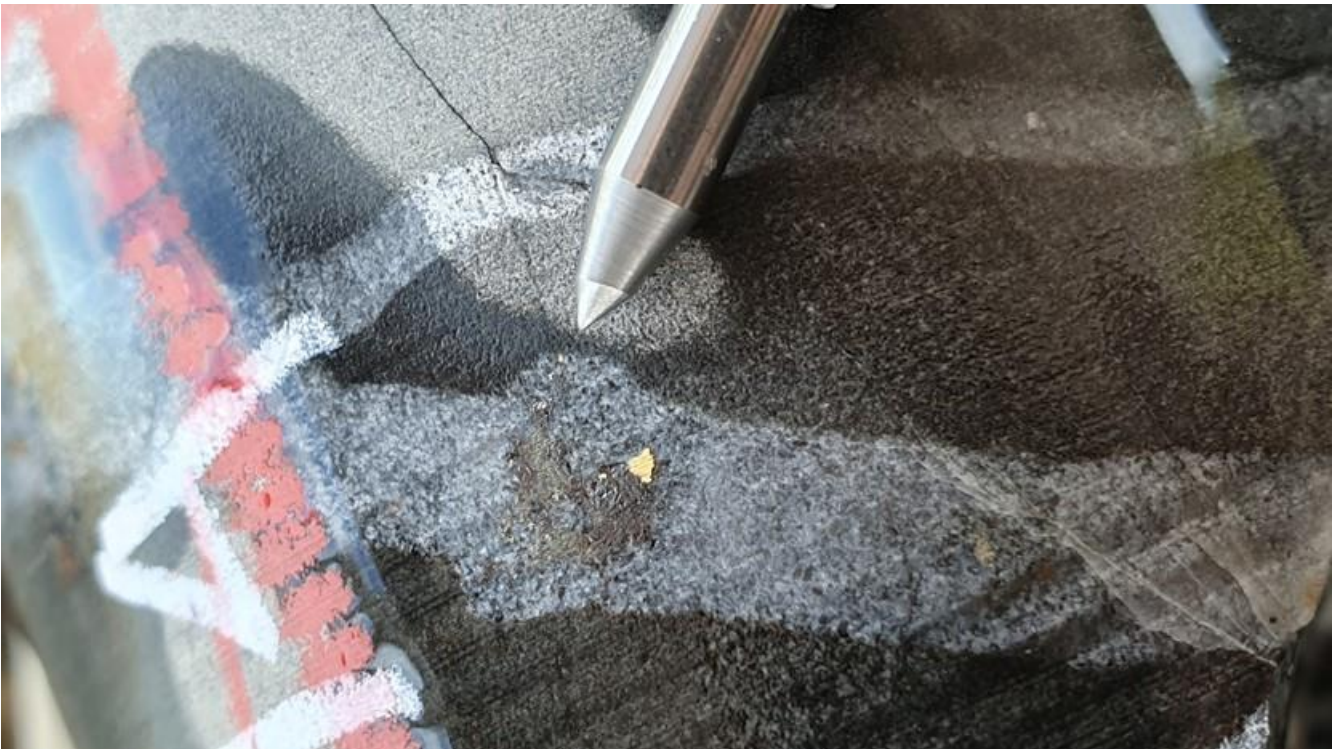
Figure 1: Visible gold identified in the Tally Ho lode at Fountain Head in FHDD181 at 174.02 grading 5.07g/t over 0.35m from 173.90m
