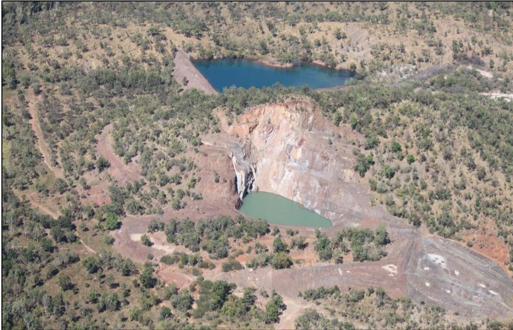
**Figure 2:** Mt Bonnie deposit aerial view (2011) looking east showing low grade stockpile in the foreground, historic open-pit centre, and water storage dam at the back of view
