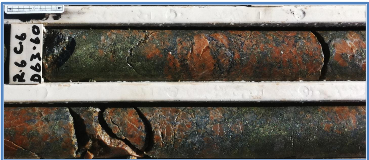
Figure 1: Chalcopyrite and Bornite in brecciated carbonate from 63.5-65.9m in PCD0040
