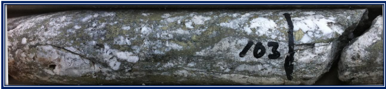
Figure 1: Chalcopyrite veins in brecciated limestone at 103m in PCD0038 (NQ drill Core 70mm diameter)
