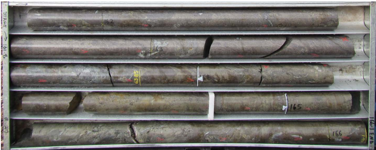
Figure 2: IBDH023 high grade massive sulphide core – the interval between 162m-165m as marked assayed 19.4% Zinc, 2.7g/t Gold, 630g/t Silver, 0.85% Copper, and 3.2% Lead
