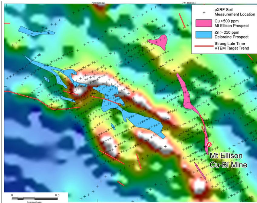
**Figure 10** Mt Ellison-Deloraine area Zn and Cu geochemistry on late-time VTEM image
