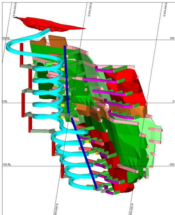
**Figure 4** Isometric view of the conceptual Iron Blow underground mine design looking south west
