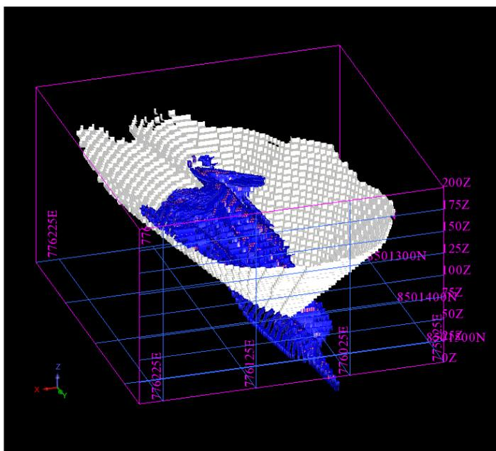
**Figure 5** Conceptual Whittle pit shell (white) for Mt Bonnie looking south, blue zone represents the orebody
